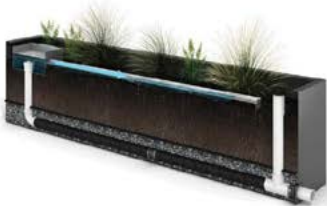
Water flows down the Level Spreader.
