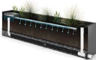
Water trickles through perforations into media.
