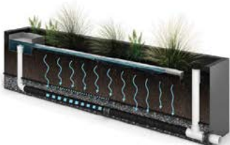
Water percolates through media and fabric.
